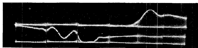
Fig. 4—Display of coupled power (top) and power transmitted past plasma in input guide (bottom) vs plasma current. Minimum current = 0.1 a; maximum current = 2.0 a.
